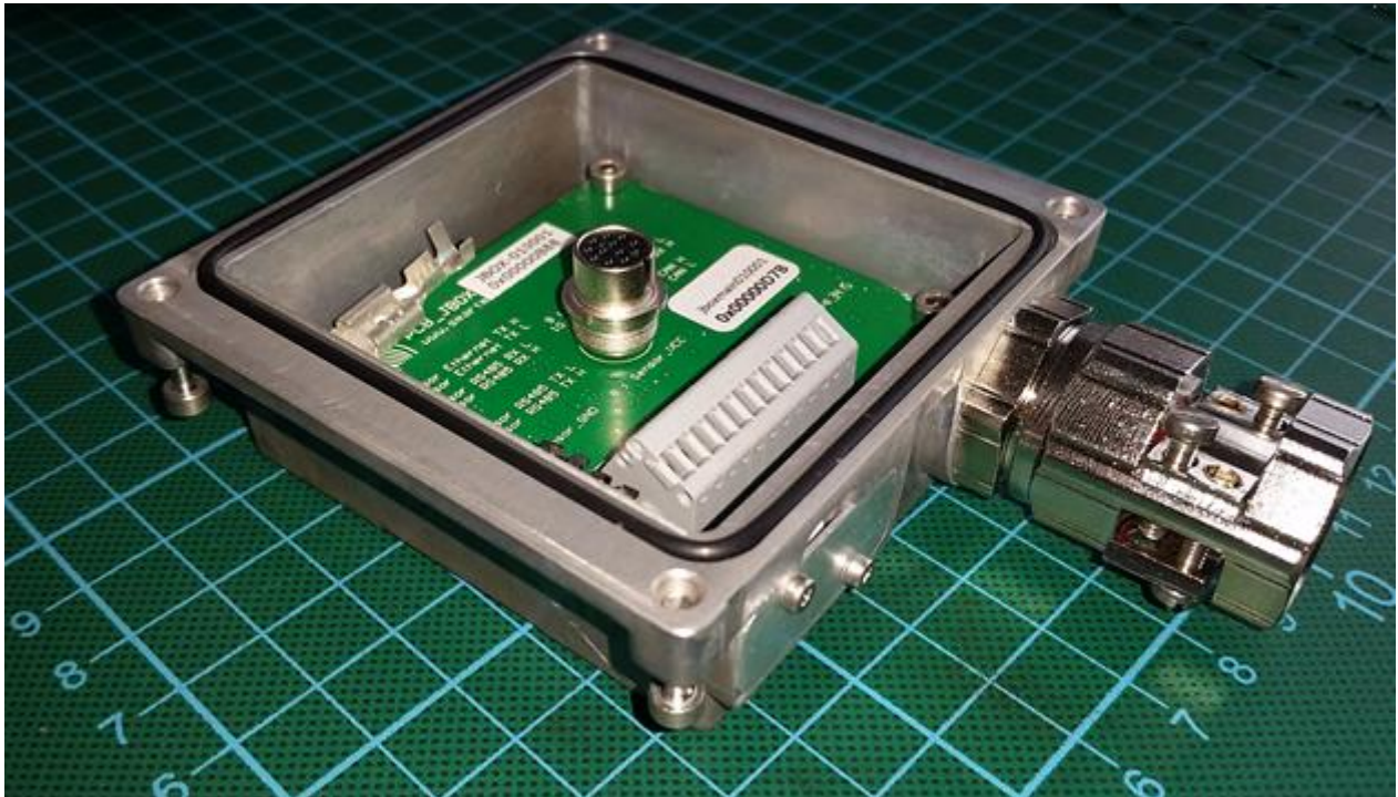
Figure 4: Junction Box JBOX-010001 inner view
