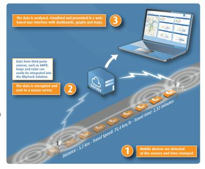
in real-time and historically. The solution is able to measure travel times on road segments with multiple flows, such as parallel train tracks, bus lanes, bike lanes and roads.
