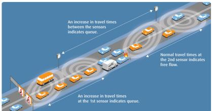
segment, unlike traditional point-based solutions with limited coverage. Real-time segment-based road monitoring provides both faster and more accurate travel times, and immediate warnings about incidents and queue. This rapid detection allows traffic managers
