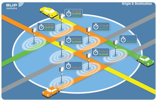
BlipTrack gives traffic engineers the ability to obtain specific and accurate statistical information about each road users' travel times, speeds, dwell times and movement patterns—from the moment they enter an area until they leave, and everywhere in between, both in real-time and historically. With this information, road authorities are able to evaluate and validate existing traffic models and plan ahead, day-by-day, hour-by-hour, and minute-by-minute.
